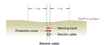
Remember drawings showing cable placement underground. If you strike a warning band or protective cover, then you are inside the safety clearance.
